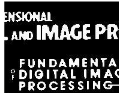
Erosion: a 2×2 square structuring element
