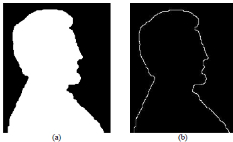
Figure 12.2 (a) Binary image. (b) Object boundary extracted using the previous equation and 3 \times 3 square structuring element.
