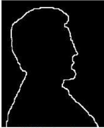
Figure 12.3 Object boundary extracted using 5×5 square structuring element
