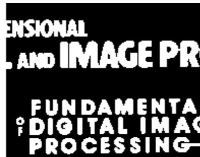
Opening: a 2 \times 2 square structuring element
