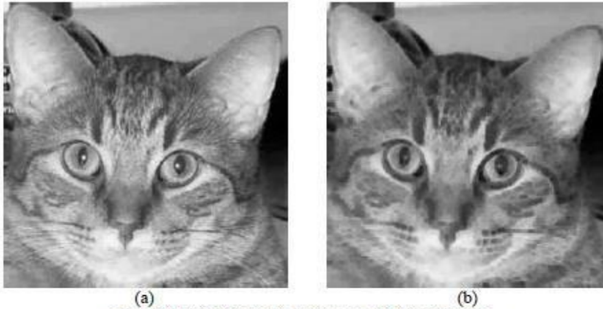
Figure 12.7 (a) Original gray image. (b) Eroded image.
