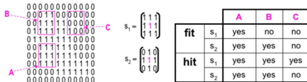
Fitting and hitting of a binary image with structuring elements s_1 and s_2 .
